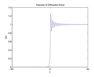
You see from the graph that the diffraction effect is most prominent near the edge of the diffraction screen (x = 0), as you expect.
