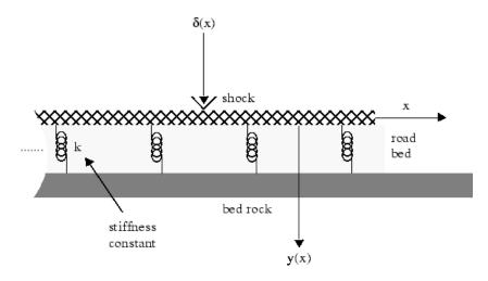
The shock could be induced by a pneumatic hammer blow.
